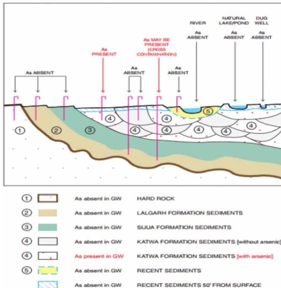
**Figure 1** | A diagrammatic geolithological sketch showing different aquifers with presence of arsenic. Diagram by Protap Chakravarti, reproduced by Sylvia Teng.
