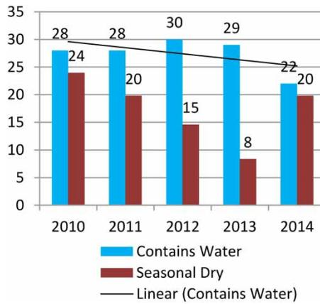
Figure 8 | Status (%) of 96 modern dugwells constructed during 2001 to 2009.
