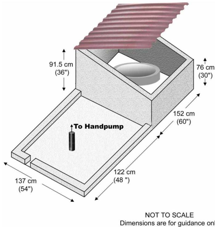
**Figure 7** | Housing – the exterior portion of the bi-tech well.
