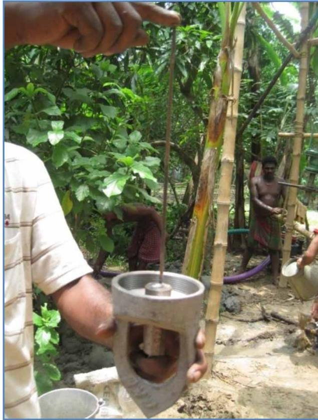
**Figure 6** | The plug fitted to close the hole of the plug cutter.
