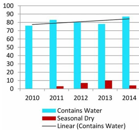
Figure 9 | Status (%) of 172 bi-tech wells constructed during 2010 to 2013.
