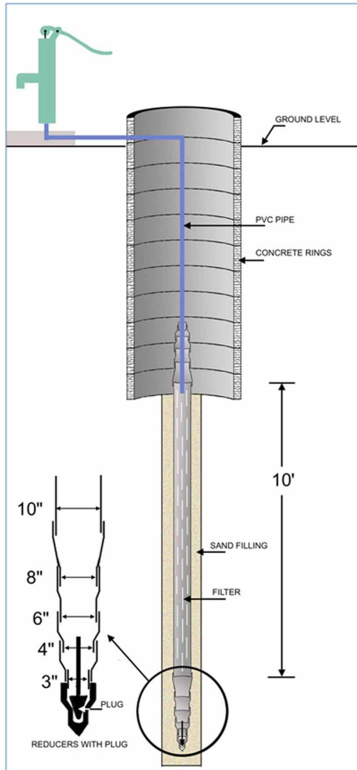
**Figure 2** | Longitudinal section of a bi-tech well.
